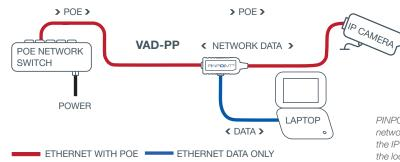
PINPOINT is inserted between the POE network and the IP camera, diverting the IP camera network connection to the local PINPOINT RJ45 port for a laptop connection.
