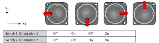
Figure.1 Mounting Orientations
