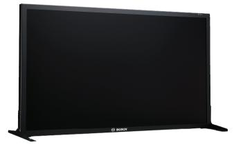
The Bosch High Performance LED monitors are high resolution color monitors ideal for use in a video surveillance environment. The monitors feature a color LCD flat-screen panel and are available with 27-inch, 32-inch, 43-inch or 55-inch viewable picture areas. Each monitor features wide horizontal and vertical viewing angles, precise color reproduction and antiimage retention.
